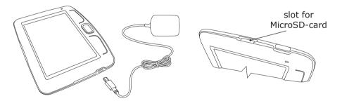
Insert SD-card into slot, as it is shown in the backside of the device. To switch the device on hold button "On/Off" **for one second.**
